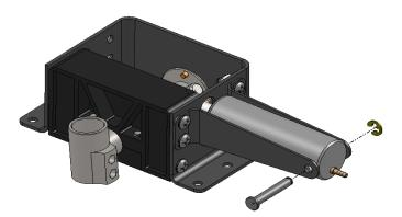
3) Remove retaining ring on cylinder piston rod and remove cylinder from assembly.
