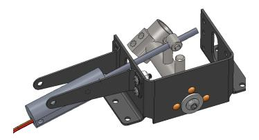
9) Locate square cam blocks onto barrel ears as shown, slide over pins in trunion
