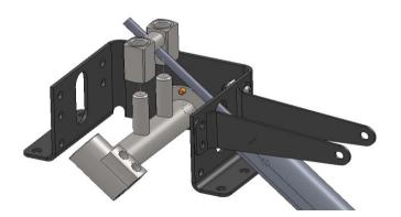
10) Spin actuator in or out to line up with mounting hole while still keeping trunion in middle position. Use provided spacers and locate as shown with clevis pin. Re-attached retaining rings.
