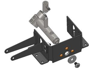
Re-assemble retrofit trunion into frame bearing with existing screw and washer. Apply Thread locker to threads.
