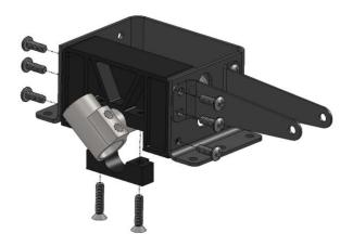
Remove trunion pivot screw, washer, and pull trunion from frame bearing. Round cam follow will be replaced by square followers included with conversion kit.
