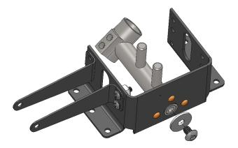
8) Slide actuator threaded rod with barrel through clearance hole in frame
