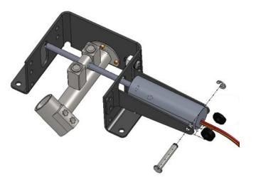
11) Locate plastic housing and trunion clamp and tighten screws.
