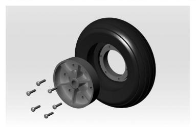
**STEP 1:** Disassemble Robart wheel by removing inner plastic wheel bearing hub from the tire. Depending upon the weight of the aircraft, Robart wheel inserts should be installed into the tire cavity for support.
