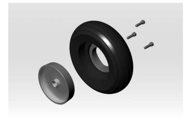
STEP 2: With the supplied machine screws (#4-40 x 1/2" SHCS), install the machined drum onto the plastic outer hub. The thru holes in the outer hub should be drilled out using a #32 or 1/8" drill. Torque the screws evenly to make sure there is a concentric and even fit. The wheel should spin true on the axle. Make sure the screws do not protrude past the drum and into the caliper area.
