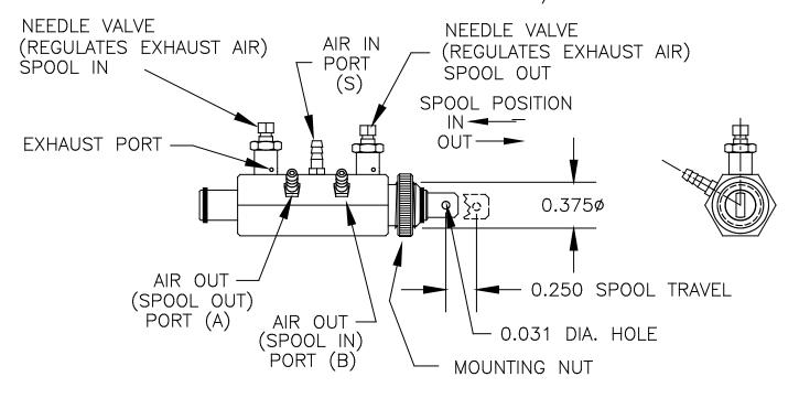
THE NEEDLE VALVE REGULATES HOW FAST THE RETRACTS MOVE.
