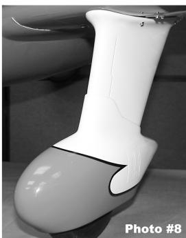
9. AFTER MOUNTING THESE ROBOSTRUT, DO NOT ATTEMPT TO FLY YOUR AIRPLANE WITHOUT FIRST CHECKING FOR THE CORRECT CENTER OF GRAVITY. These RoboStruts add about 9 oz.. to the weight of the airplane and will change your actual center of gravity if your airplane was set up for the wire gear.
