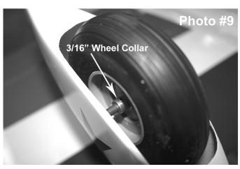
8. After you have the wheel installed on the strut and wheel pant remove the axle and grind a flat spot on it and reinstall the axle and make sure you use blue threadlocker on all of the set screws.
