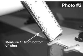
3. Remove wire from wing and cut the wire with a Dremel® tool and cutoff wheel at the 1 inch mark, (See photo #3) after cutting deburr around the edges of the wire so that there are no burrs on the wire. This will elminate difficulties on putting the strut over the wire.
