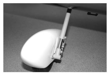
10. AFTER MOUNTING THESE ROBOSTRUT, DO NOT ATTEMPT TO FLY YOUR AIRPLANE WITHOT FIRST CHECKING FOR THE CORRECT CENTER OF GRAVITY. These RoboStruts add about 7 oz. to the weight of the airplane and will change your actual center of gravity if your airplane was set up for the wire gear.
